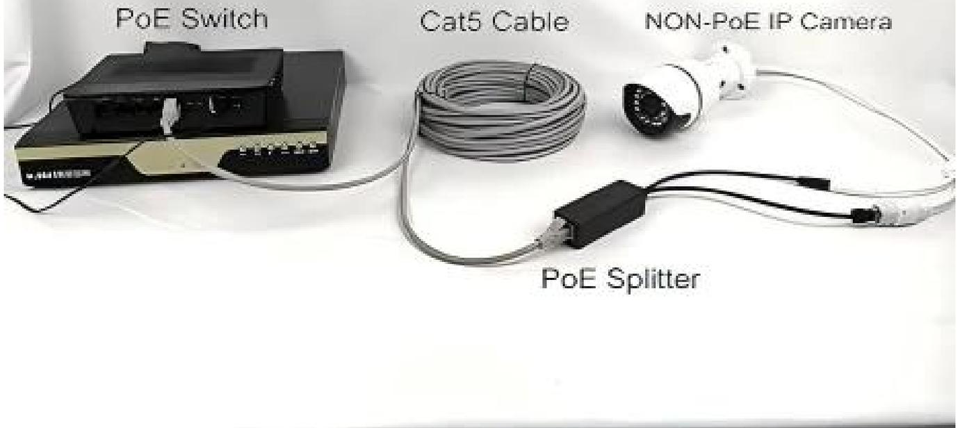
The **POE** 12V 1.2A 13.5W IEEE 802.3AF POE 5.5 x 2.1mm 12V DC POE RJ45 IP NVR AP IoT
