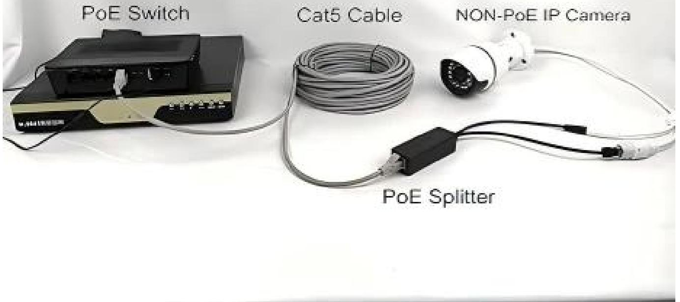
POE 12V 1.2A 13.5W IEEE 802.3AF POE 5.5 x 2.1mm 12V DC POE RJ45 IP NVR APS IoT
